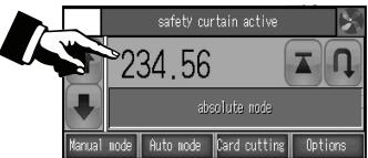
To input the required dimension, press the dimension on the screen and input the value via the on-screen keyboard.
