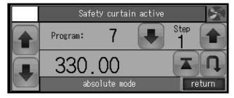
The dimension where the cut was made is saved automatically as a step dimension in the current program. After each cut, program automatically moves to the next step.
