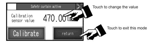
When starting the cutter, measure the cut paper and compare that measurement with the on-screen display. If both dimensions do not match, the operator must adjust the base dimension, following these steps:
