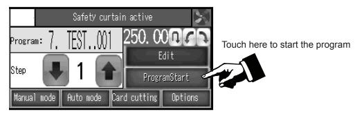
After pressing Program Start, the back gauge moves to the dimension saved in step 1 and a new screen appears:
