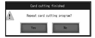
Pressing **YES** moves the back gauge automatically into the first dimension to repeat the same program. Pressing **NO** exits the program.
