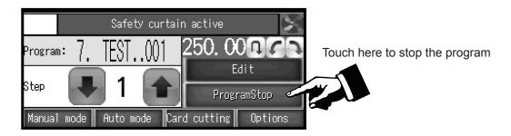
After each cut, the back gauge moves to the next step. When the last cut is made in the selected program, the back gauge automatically returns to Step 1 and the program can be repeated.
