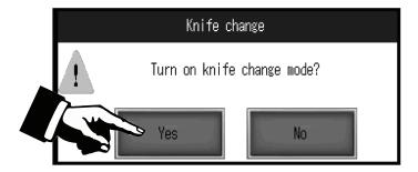
Press **YES** and make a cut by pressing the two cut buttons on the front of the cutter. This will put the knife in the lowered position, ready to be changed. Change the knife according to instructions in Operator/Maintenance Manual.
